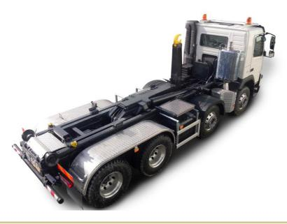
Innovative concept with tilting frame that is locked on the sub-frame in loading phase
